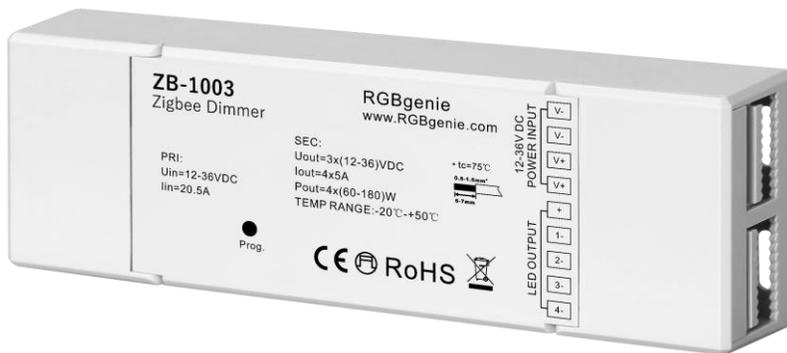
The ZB-1003 is a ZigBee enabled 4 channel LED Controller utilizing the latest ZigBee 3.0. With a 12 to 36 volt DC input, this robust unit provides up to 720 watts of constant voltage power up to 5 amps per channel for maximum lighting compatibility.
